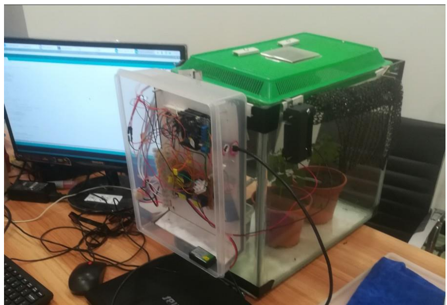
Fig. 17. Setup for Controlling a Greenhouse using Sensors for Optimum Growth of Plants
